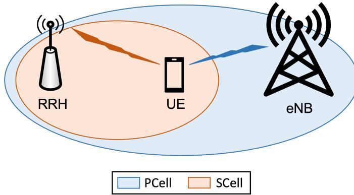
Figure 2.9: Inter-site carrier aggregation.
