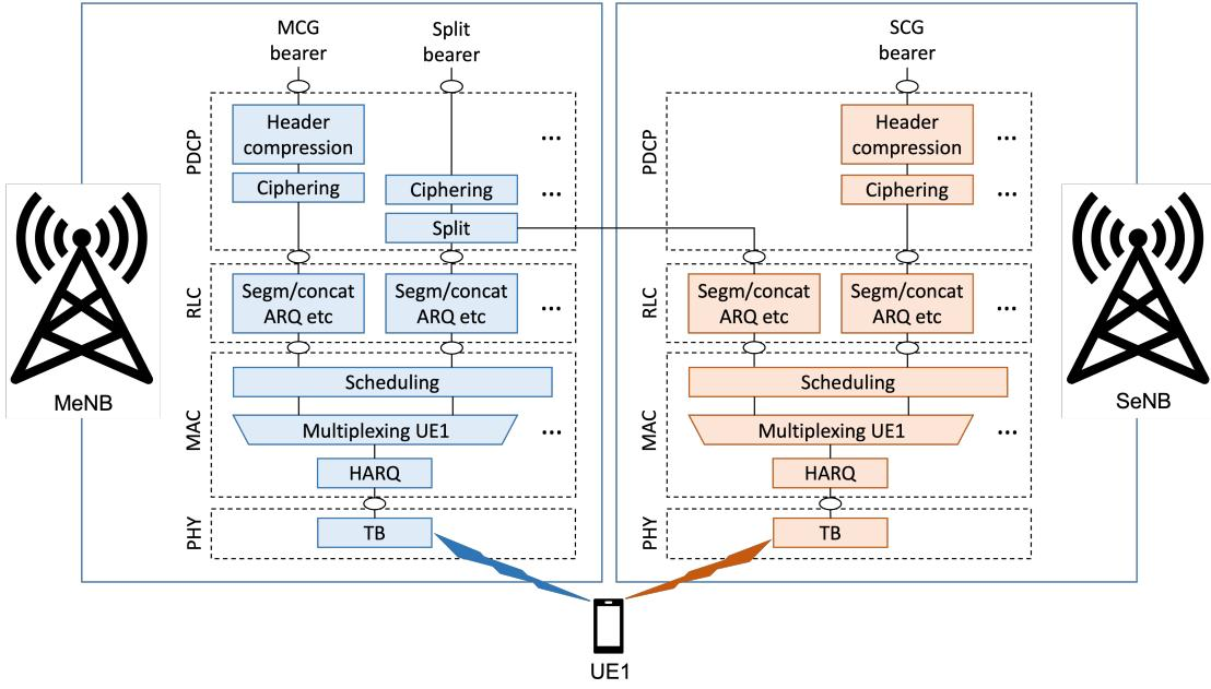
Figure 2.12: Layer 2 structure for DC in LTE.
