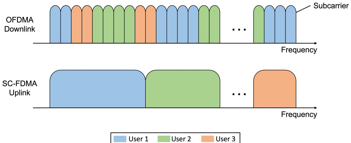
Figure 2.4: LTE multiple access technologies.
