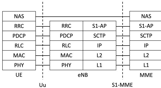
Figure 2.3: LTE protocol stack - Control plane.
