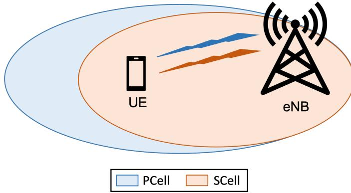
Figure 2.7: High-level CA diagram.
