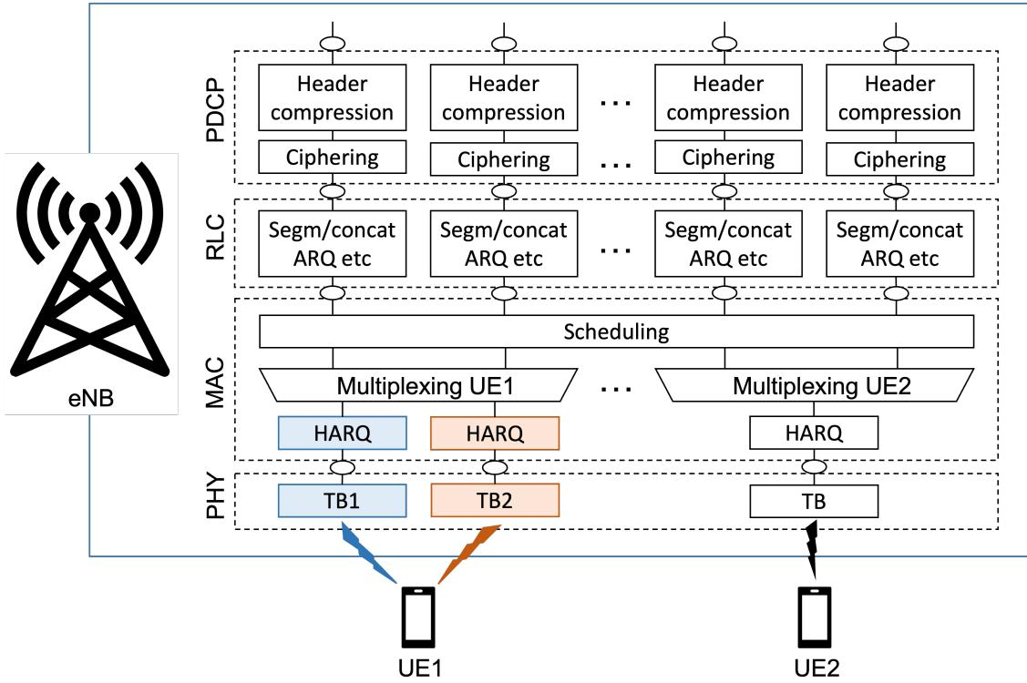
Figure 2.8: Layer 2 structure for CA in LTE.
