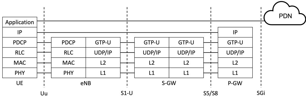
Figure 2.2: LTE protocol stack - User plane.
