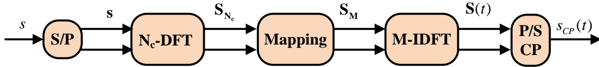
Figure 4.1: Transmission scheme in SC-FDMA
