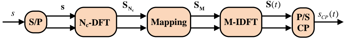
Figure 2.3: Transmission scheme in SC-FDMA
