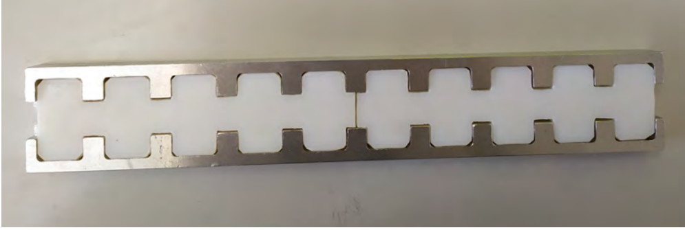
Figure 5.3: Aluminum cavity filled with the 3D-printed dielectric to assemble the array.
