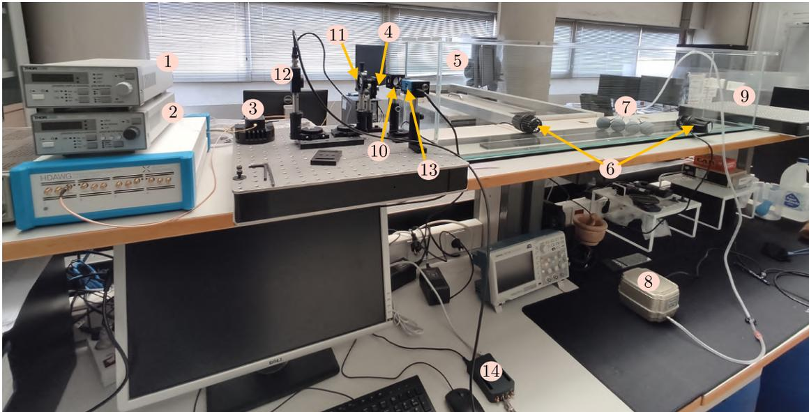
(b) Actual implementation of the UOWC experimental system setup.
